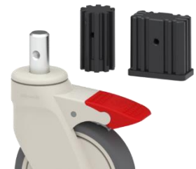
Quick and hassle-free installation with plastic adaptors that would fit easily into the pipe of bed legs. Available in round shape (ø27,3mm, ø28,5mm, ø29,3mm, ø35,5mm and ø39mm) and rectangular shape (27mm × 57mm and 36 × 36mm). Applicable only to castors with SF20 suffix.
